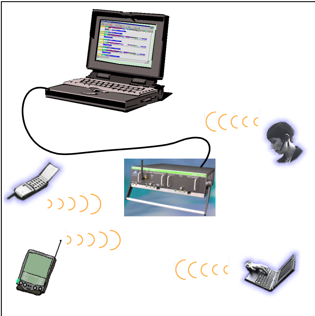
Sample Bluetooth Piconet with BTTracer Protocol Analyzer
